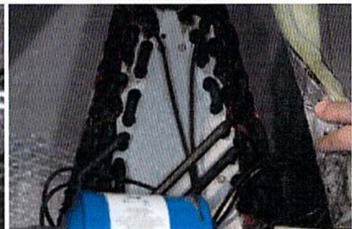
Sulfide corroded coil
